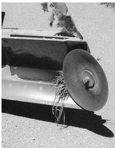
(1) The Gravel Saver disk in place on moldboard.
