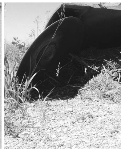
(2) Closeup view of the disk blade moving gravel.
