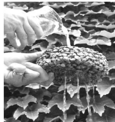
**Figure 2: Pervious Concrete<sup>7</sup>**
